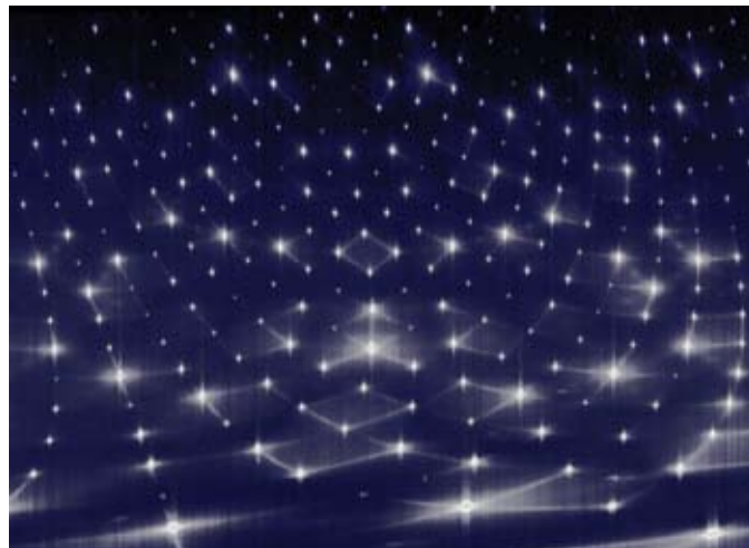
From Branton Campbell: Diffuse scattering distribution concentrated in the L = 5 plane of a natural single-crystal sample of zeolite mordenite. This Weissenberg-like image was extracted from a series of CCD images collected at beamline 33ID-D (20 keV) of the Advanced Photon Source. Three distinct features are evident: broad hazy patches, open diamonds, and star-shaped distributions around each Bragg peak. Each reveals an important component of what turns out to be a complex fault-defect architecture with implications for mordenite's adsorptive and catalytic properties. B. J. Campbell et. al., J. Appl. Cryst. (2004). 37, 187-192.
