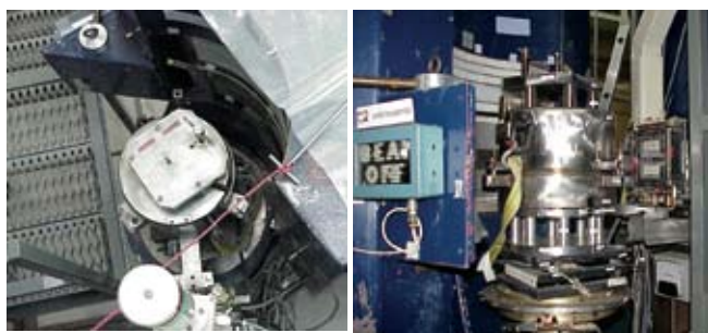
(left) bird's-eye and (right) side views of the loaded AECL shielded cell on the NRC C2 neutron powder diffractometer
