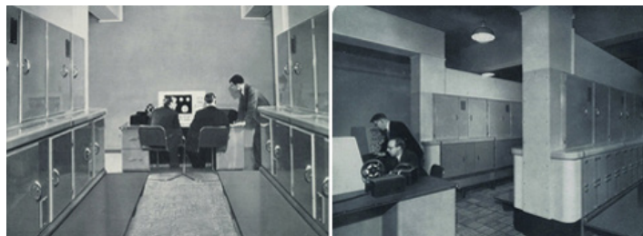
A Ferranti Model No. 1 computer of the 1950s installed at the U. of Manchester, UK
