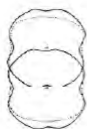
Shape of the effective atom-atom potential in solid chlorine; broken line: effective shape of the atoms in the crystal
