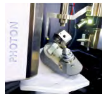
An Almax Easy Lab diamond anvil cell (DAC) suitable for x-ray diffraction mounted on the Kappa goniometer of the Bruker D8 Venture instrument at UNF
