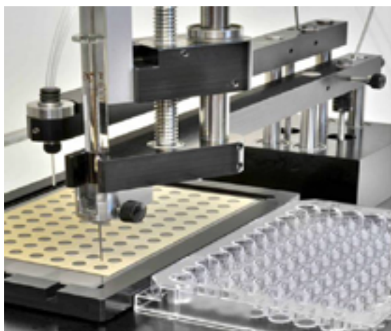
Dispensing LCP to "sandwich" plates
