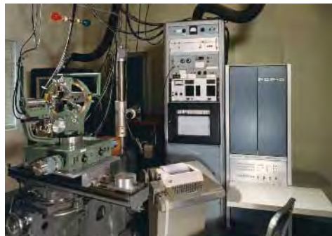
Fig. 2: The four-circle Picker x-ray diffractometer and the PDP-5 computer that was programmed to control it (Photographs courtesy of ORNL)
