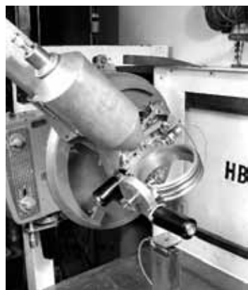
Fig. 1: The three-circle paper-tape controlled neutron diffractometer. (Photograph courtesy of ORNL).
