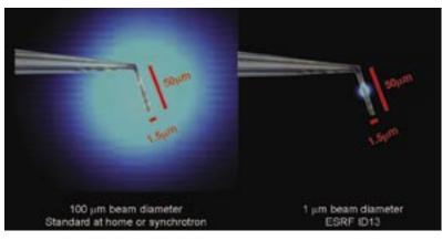
Comparison of beam sizes relative to a crystal of the fibril-forming peptide from yeast prion Sup35. The crystal is mounted on the end of a glass fiber, frozen in a cold nitrogen gas stream, and viewed along the x-ray beam on ESRF beamline ID-13. The beam is viewed on a fluorescent detector mounted downstream of the crystal.
