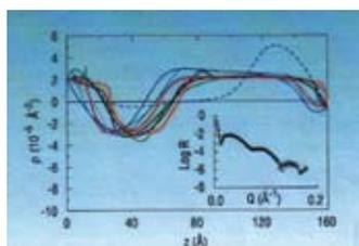
To help explain the flow diagram, the figure at left illustrates the ambiguity that can result in the scattering length density profile extracted from a single set of reflectivity data (insert at lower right). The film structure is that of TiO on Ti. The family of solid curves for the scattering length density profile generate a fit to the measured reflectivity data that is as good as that obtained for the dashed curve!
