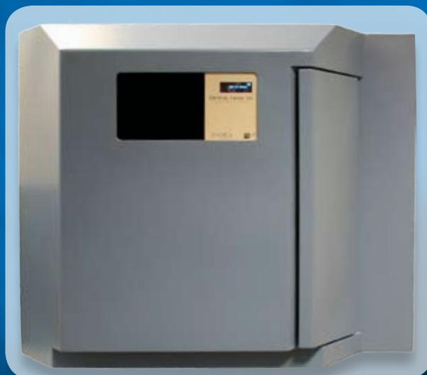
The Crystal Farm Imaging System combines both incubation and imaging for the ultimate crystal plate storage and retrieval tool which simplifies the protein crystallization process.
