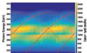
Measurement of sulfur L2,3 and carbon K edge XANES in a polythiophene film using a high harmonic supercontinuum
