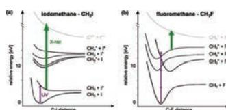
Charge transfer in dissociating iodomethane and fluoromethane molecules ionized by intense femtosecond X-ray pulses
