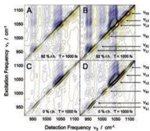
Ultrafast vibrational dynamics of the DNA backbone at different hydration levels mapped by two-dimensional infrared spectroscopy
