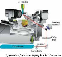
Apparatus for crystallizing ILs in situ on an X-ray diffractometer
