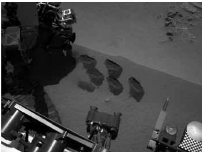
NASA's Mars rover *Curiosity* used a mechanism on its robotic arm to dig up five scoopfuls of material from a patch of dusty sand called "Rocknest," producing the five bite-mark pits visible in this image from the rover's left navigation camera (Navcam). Each of the pits is about 2 inches (5 centimeters) wide.
