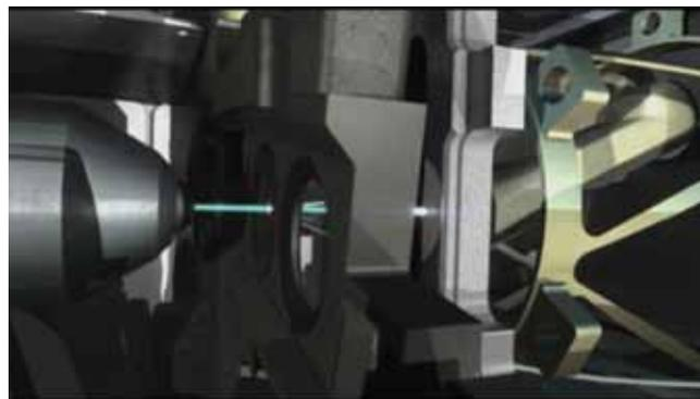
CADview image of the inner workings of the CheMin diffractometer. The x-ray source is on the left with a beam of x-rays intersecting the mineral grains in the sample chamber and the diffracted beams going to the detector on the right.
