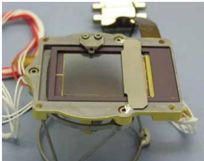
This charged coupled device (CCD) is part of the CheMin instrument on NASA's *Curiosity* rover. When CheMin directs x-rays at a sample, this imager, the size of a postage stamp, detects both the position and energy of each x-ray photon. The technology in this CCD was originally developed by NASA and has become widely used in commercial digital cameras and other imaging devices. *Image credit: NASA/JPL-Caltech/Ames.*
