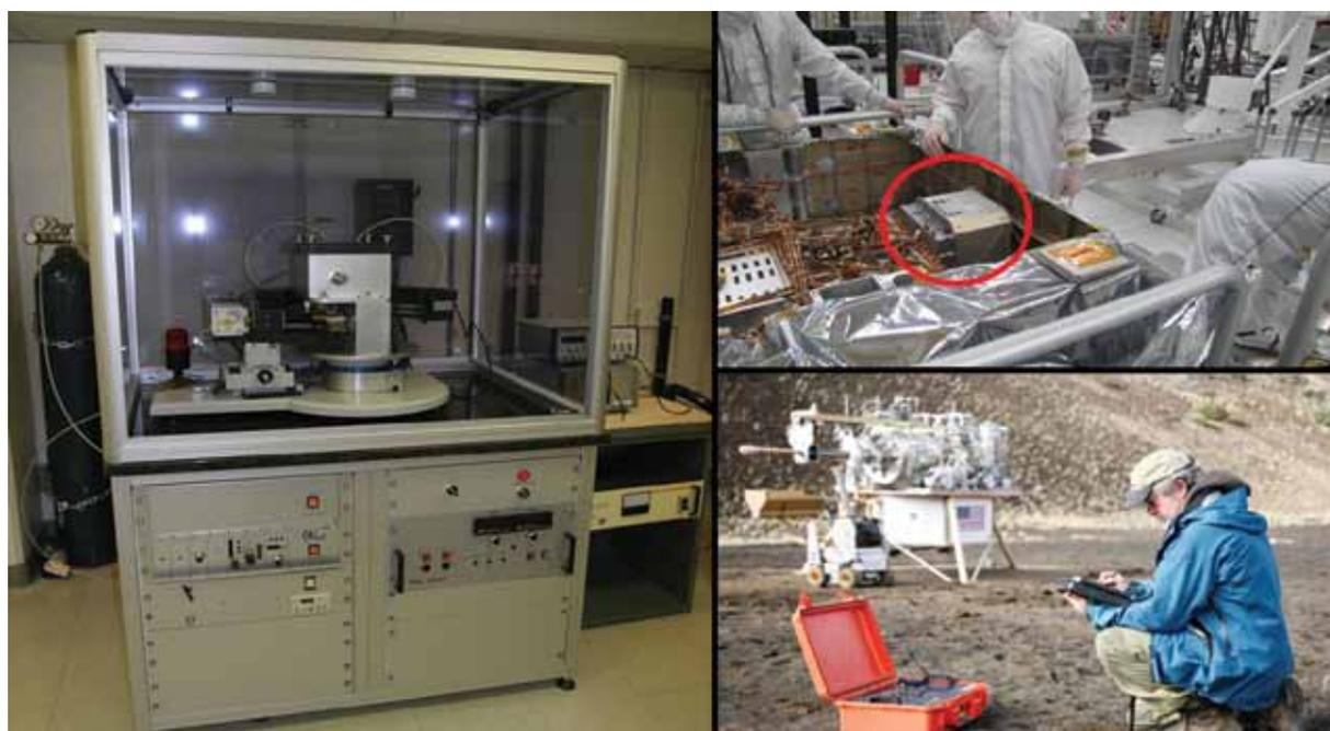
On the left is a typical powder diffractometer. The upper right is an image of the rover while it is being assembled, indicating the CheMin instrument in its place. The lower right shows Dave Blake using the briefcase sized version of the instrument.
