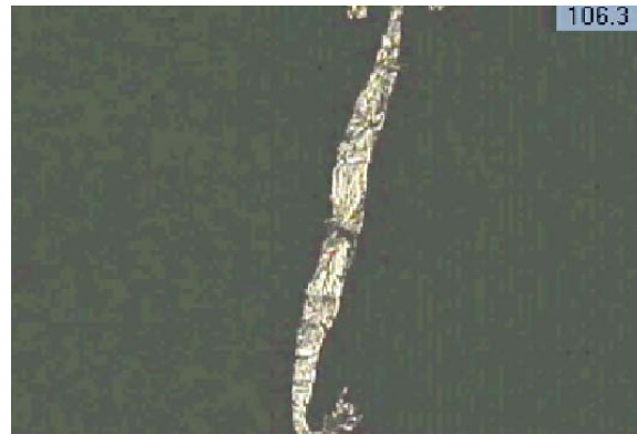
Figure 9. Some observations of the mixed fusion behavior of malic acid. The two sides of the sample are the two enantiomers of malic acid. The high melting cocrystalline phase is racemic malic acid.
