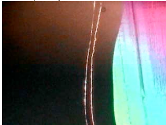
Figure 10. The mixed fusion behavior of the catechol (left) / p -phenylenediamine system.
