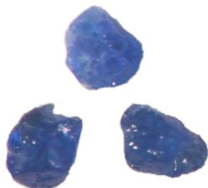
**Figure 3.** Optical image of single crystals of  $\text{Ba}_3[(\text{VO})_2(\text{C}_2\text{O}_4)_5(\text{H}_2\text{O})_6]\cdot(\text{H}_2\text{O})_3$ . Crystals are  $\sim 0.5$  mm in length.
