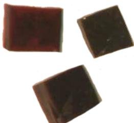
**Figure 1.** Optical image of single crystals of  $\text{Cs}_2\text{V}_3\text{O}_8$ . Crystals are  $\sim 0.2$  mm in length.
